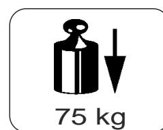
$$D = \frac{\text{MAX KG} \times \text{MAX KG}}{\text{MAX KG} + \text{MAX KG}} \times 0,00981 \leq 7,52 \text{ kN}$$
